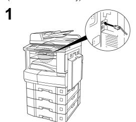
Connect the printer to the PC with an USB cable.
