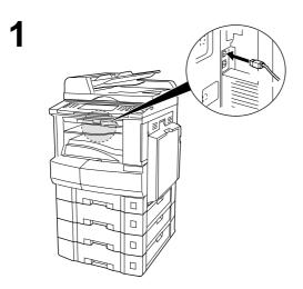
Connect the printer to the PC with an USB cable.
